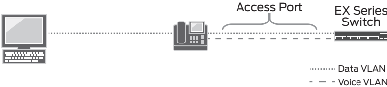
Figure 4.4 Switch Port Configured as an Access Port With Voice VLAN, IP Telephony, and PC Sharing the Same Switch Port
