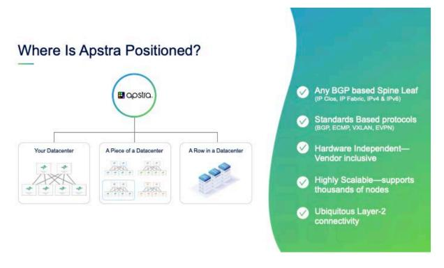
The data store collects and analyzes device telemetry, which enables Apstra to identify anomalies, report on impacts (for example, packet loss or device failure), and identify the root cause of problems. Network engineers can allow Apstra to remediate problems automatically, or to share root cause analysis with engineers to speed up manual remediation.
