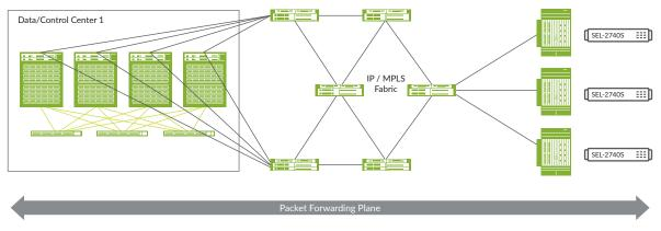
Figure 2: Solution requirements components for the packet-based forwarding plane
