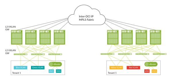
Figure 3: Single fabric, geo-redundant data center
