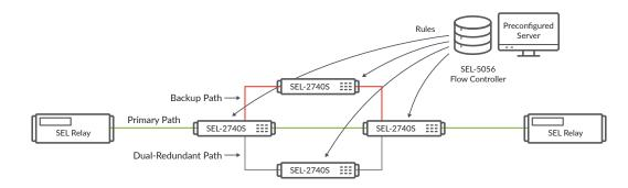
Figure 4: SEL Inc.'s OT-SDN Ethernet fabric
