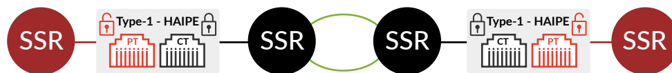
Figure 2: Mission planners can create a double-bookended network with secure vector routing. The SSRfC architecture combines secure vector routing with domain-specific features of the Juniper Session Smart Router to create a double-bookended secure routing architecture that provides IPsec-based encryptors (HAIPE or CSfC) with greater visibility and control than previous approaches.
