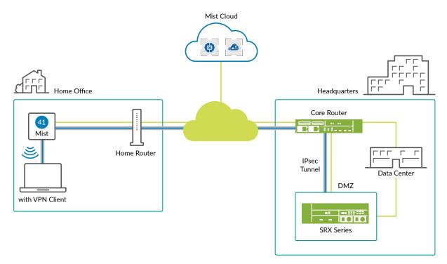
Figure 1: Mist Wi-Fi for Remote Workers solution
