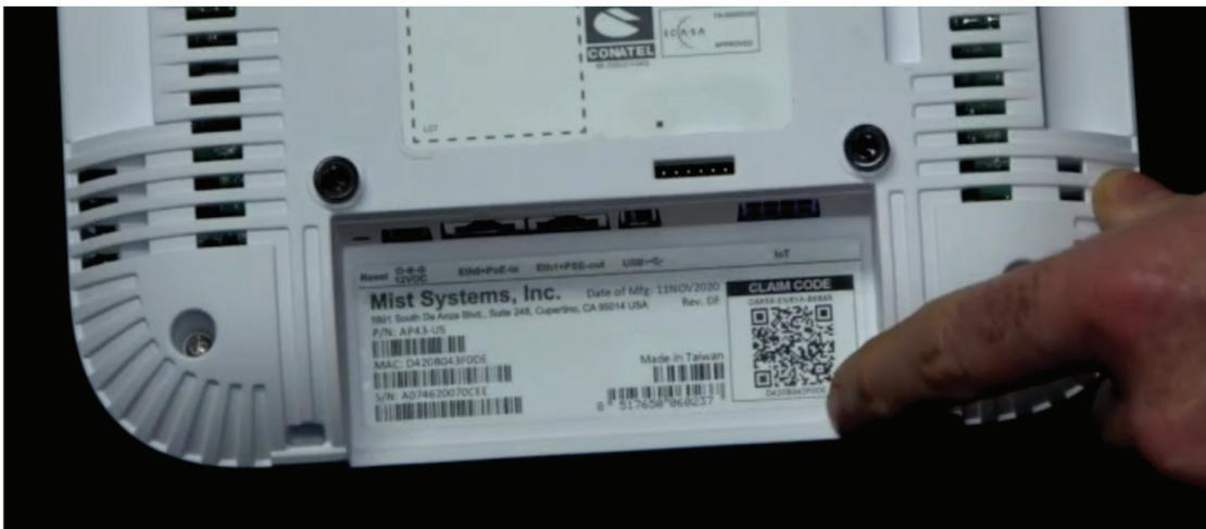
Figure 27: QR Code on an Access Point
