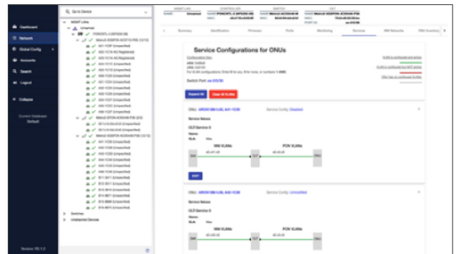
Figure 4: GUI windows from PON Manager: OLT data, ONU/ONT administration, and service provisioning
