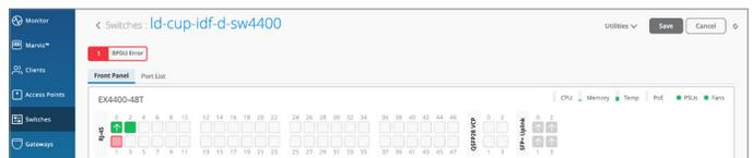
Figure 8: Wired Assurance BPDU Guard error
