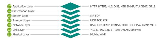
Figure 6: Supported protocols by OSI layer
