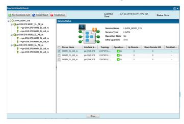
Figure 4: Functional Audit—control plane and data plane validation
