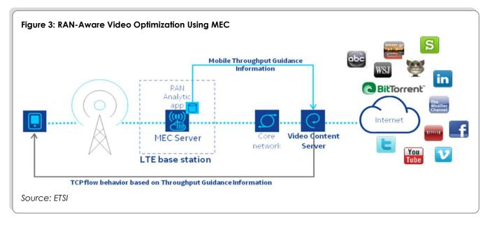
The idea is to use a RAN analytics application to determine/estimate the throughput likely to be available at the radio downlink interface for a user, and then use packet headers to convey that information to the video server, so that it can adapt the stream accordingly. Field trials have shown noticeable performance improvements when operators communicate RAN conditions to the video server in this way.
