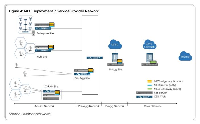
In the macro cellular network, good candidates for MEC deployment are preaggregation or hub sites, which concentrate approximately 20-30 cell sites and enable a round trip latency to and from the base station of approximately 3-5 ms. Larger aggregation sites, which concentrate 100 or more cell sites, are also attractive, and even though this may result in higher latency, it would still be still lower than for services deployed "behind" the centralized core.
