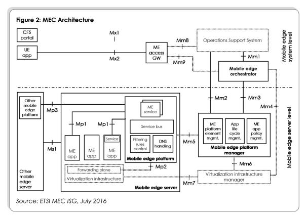
Adopting the ETSI MANO model makes the MEC infrastructure an open environment that will allow the operators to deploy applications and services from third-party vendors. This makes interoperability important and, because it is a distributed deployment, places a great emphasis on low cost of operations. A standardized NFV Infrastructure (NFVI) platform connected by an SDN-enabled network is important to this realizing this goal.
