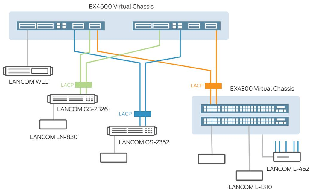
Figure 1: Juniper Networks and LANCOM Systems wired and wireless collapsed campus solution
