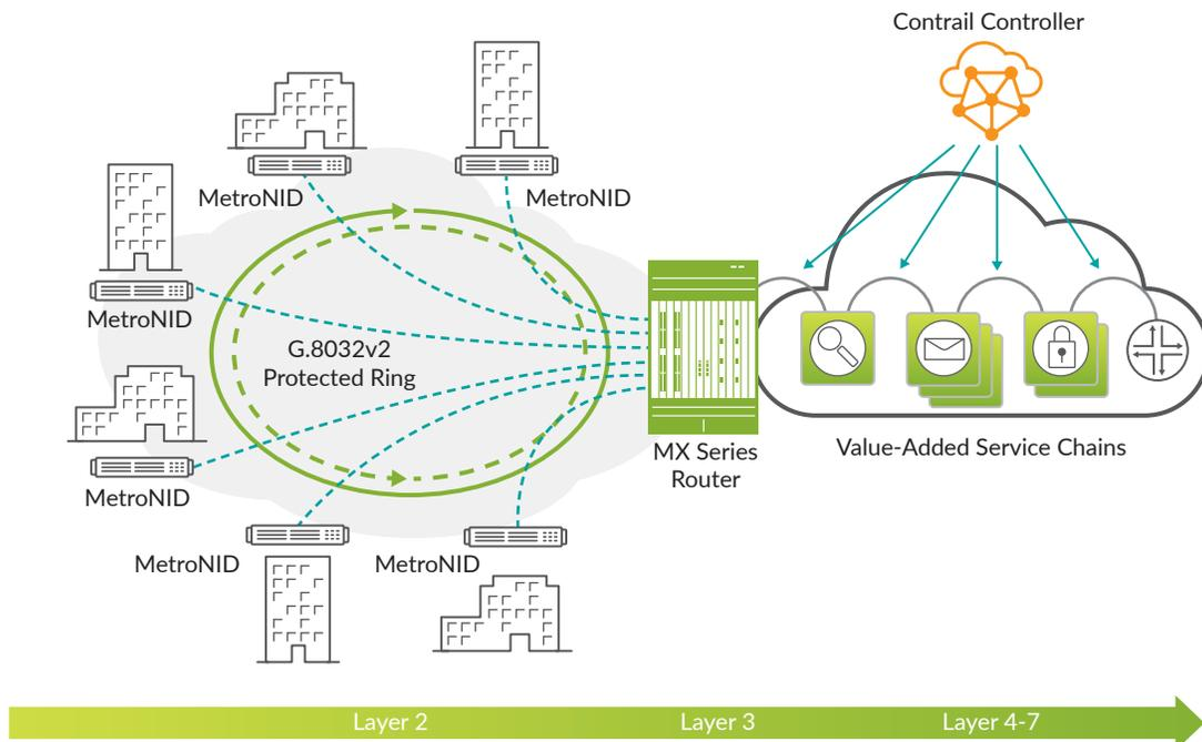
Figure 2: Juniper and Accedian Networks' joint solution
