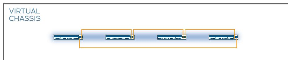
**Virtual Chassis Fabric** (VCF) evolves Virtual Chassis by allowing customers to interconnect multiple switches into a spine-and-leaf fabric architecture and manage the interconnected switches as a single device. VCF provides many of the benefits of a Virtual Chassis while supporting up to 20 devices. VCF works well for small data centers in which the Point of Delivery (POD) size could be as large as 16 racks, and can still be managed from a single device for the entire fabric.
