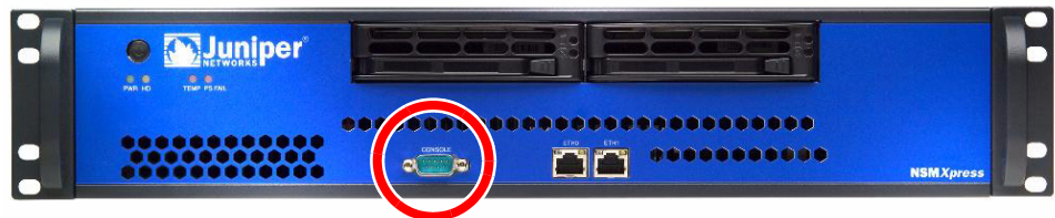
Figure 3: The console port is located on the front panel
