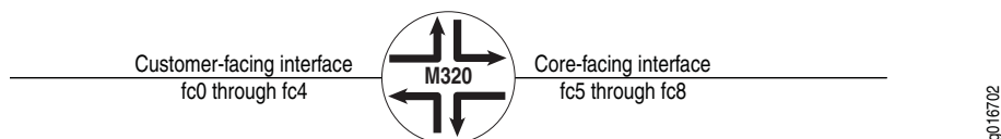
Figure 6: Customer-Facing and Core-Facing Forwarding Classes
