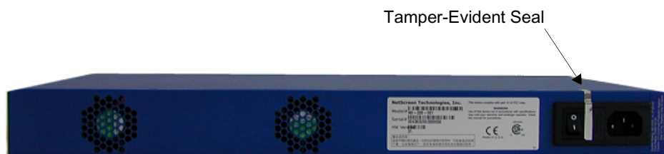
Figure 1 Tamper-Evident Seal on AC Interface
