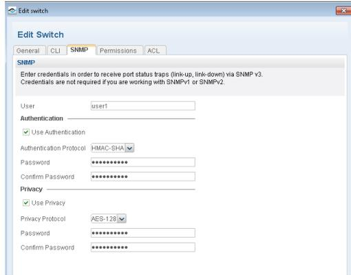
Figure 7: Device configuration (switch page shown) - SNMP information
