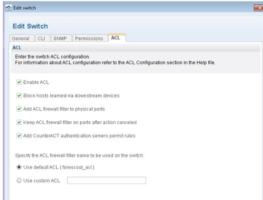
Figure 9: Switch-Device configuration (switches only) - ACLs
