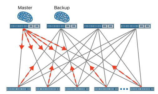
Figure 4: Virtual Chassis Fabric integrated control plane
