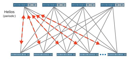
Figure 3: Autodiscovery with Virtual Chassis Fabric technology
