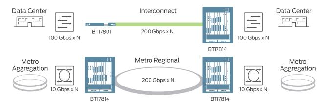
Figure 1: BTI7800 flexible, scalable deployment options
