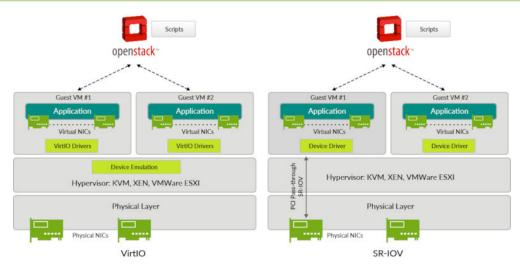
Figure 1: The vMX architecture for VirtIO and SR-IOV.
