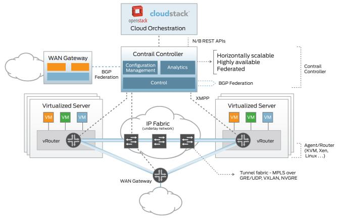
Figure 1: Contrail components for automating and orchestrating creation of virtual networks
