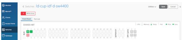
Figure 11: Wired Assurance BPDU Guard error
